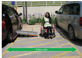
Wide Access Aisles Versus Narrow Access Aisles The photo above shows a van-accessible space, which is next to a wide (eight foot) access aisle. The wheelchair user needs this much space, at a minimum, to safely lower the ramp and exit or enter the van.
