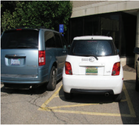
Access aisles are not intended for emergency parking, as shown in the violation above.
